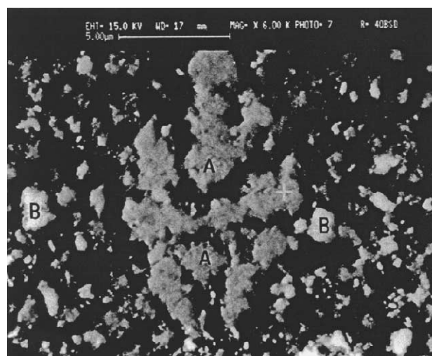
Fig. 9. SEM photograph of a catalyst pellet showing the middle section of the catalyst bed ( \times 6000 ): (A) rich in oxygen and lean in carbon; (B) rich in iron.
